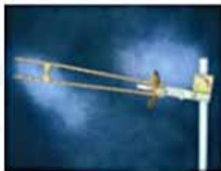
Yagi antenna 17 dBi gain
